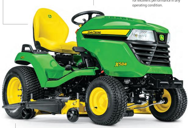
**Four-wheel steering.** All four wheels on the X584 steer the tractor for ultimate trimmability.
